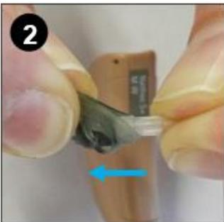
Remove the dome by pulling on its edge.
