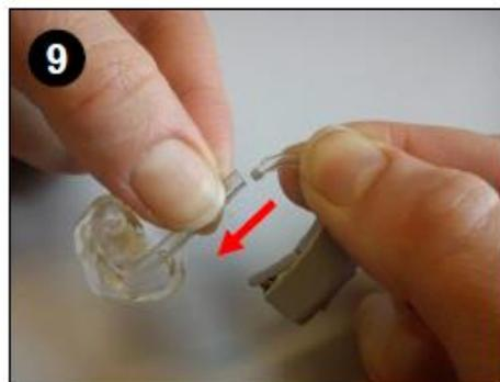
**9** Finally push the hearing aid back onto the tubing.
