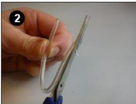
Cut a taper into one end of the new tube using scissors. Some tubes come pre-tapered.
