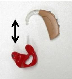
Gently pull the soft tubing off the hooked part of the aid by holding on to the tubing and the hook of the aid and tugging gently. Don't pull it out of the ear mould as you won't get it back in again.
