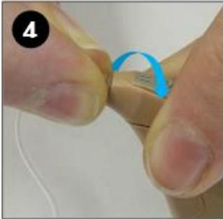
Now unscrew the thin tube from the hearing aid itself. It's probably easier to firmly grip the end of the tube and rotate the hearing aid.
