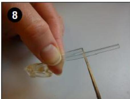
**8** While still holding the old tube over the new, cut the new tube to the correct length. Make it very slightly longer as you can always trim a little more off.
