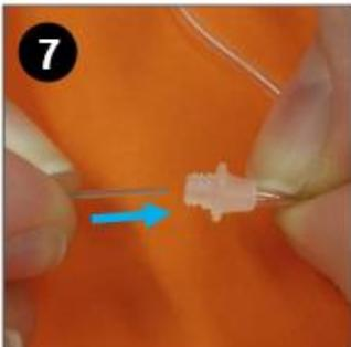
Now push the green wire down the tube from the side that was attached to the hearing aid.
