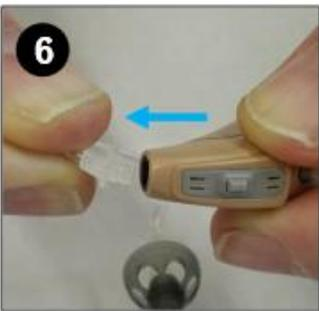
Remove the thin tube from the hearing aid.
