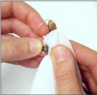
Clean the dome and the speaker unit with a wet wipe or slightly damp cloth. Make sure it is not too damp as this could damage the speaker.
