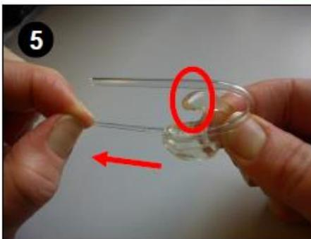
Pull the tube through until you reach the bend in the tube. Notice the top part of the tube is in line with the tip of the prong at the top of the mould (circled in red).
