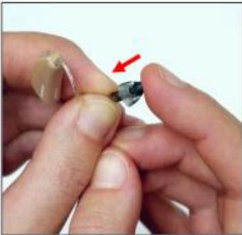
Push the new dome onto the speaker.
